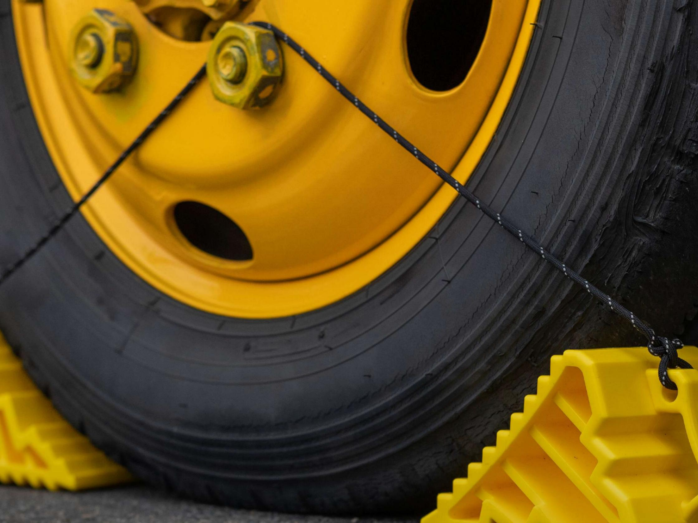
A close-up photograph of a yellow wheel with a black tire. A black rope is tied around the wheel and extends to a yellow wheel chock on the ground. The chock is a bright yellow, stepped plastic device used to immobilize a vehicle. The background is a dark, textured surface, likely asphalt or concrete.
